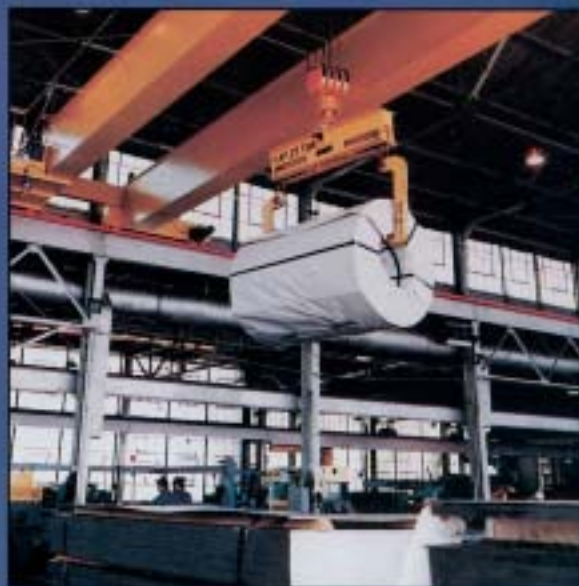
This 25 ton coil handling crane in a steel service center is a typical application for a custom-engineered hoist.
