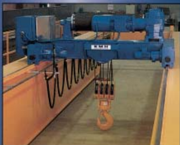
This 25 ton coil handling crane in a steel service center is a typical application for a custom-engineered hoist.
